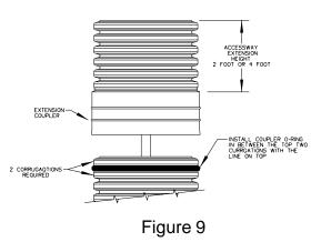
11. Attach the vent pipe extension with the 2" vent coupling, bringing the vent well above grade.
