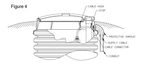
Supply Cable Voltage Drop: 120 VAC Pump = .195 Volts per Foot of Cable 240 VAC Pump = .098 Volts per Foot of Cable (Maximum Recommended Length = 100 Feet)
