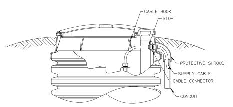
Power at the station must not drop below 10% of nameplate voltage. Maximum Recommended Length: 120 Volt 60' (min. voltage at pump — 108V) 240 Volt 150' (min. voltage at pump — 216V) Consult factory for longer lengths
