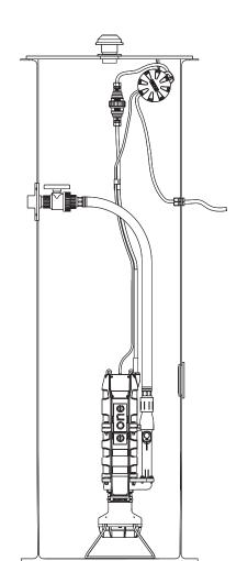
The model GH091 (Gatorgrinder) grinder pump station is a complete unit that includes: the grinder pump, check valve, fiberglass tank, controls, and alarm panel. Designed specifically for installation in warmer climates, the Gatorgrinder is an efficient, economic station for single dwelling service.
