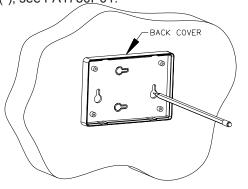
Mount the back cover to the wall. Run the cable through one of the holes in the cover. Do not connect the cable to the e|one Sentry yet.
