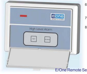
Run a 2-conductor, 18-22 AWG electronic signal cable that is UL-rated for 300 volts from the alarm panel to the wall location of the E/One Remote Sentry. Connect the cable to the contacts for Remote Sentry or to Dry Contacts (DC) in alarm panel. (Note: If DC's are used, the Remote Sentry will not work in a power loss situation) Note: This connection has no polarity, unless connecting to an Indoor Unit (IDU), Red = (+), Black = (-), see PA1730P01.
