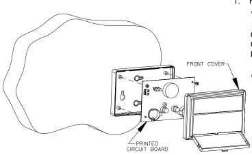
2. Disassemble the E/One Remote Sentry enclosure by snapping off the front cover. Remove the 4 screws securing the printed circuit board and remove circuit board.
